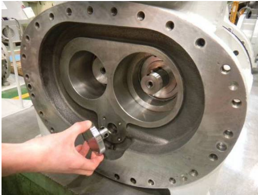
Photo 054 Removal of Oil Injection Pipe Retainer
