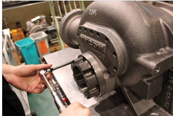
Photo 029 Removing High-stage Unloader Cylinder
