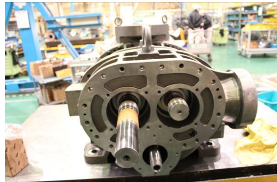
Photo 052 Bearings are Just Removed
