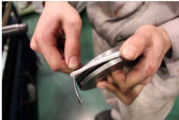
Photo 030 Removing the Cap Seal of the Unloader Piston
