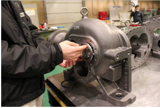
Photo 074 Attaching O-ring Spacer (High-stage)
