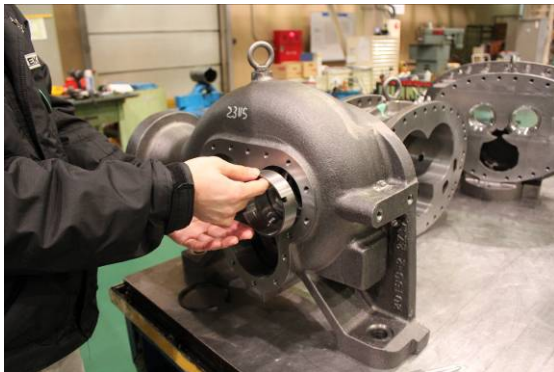
Photo 076 Attaching Balance Piston Sleeve
