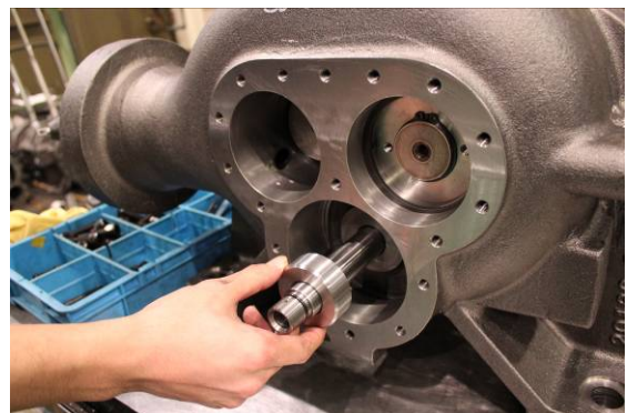
Photo 086 Attaching Load Capacity Adjustment Spacer (Spacer for 20% Load)
