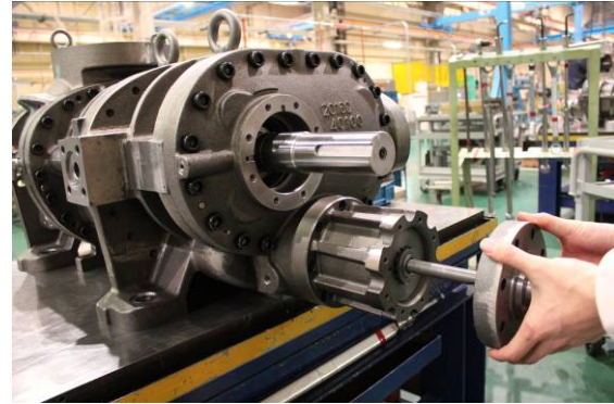
Photo 022 Removing Unloader Cylinder Cover
