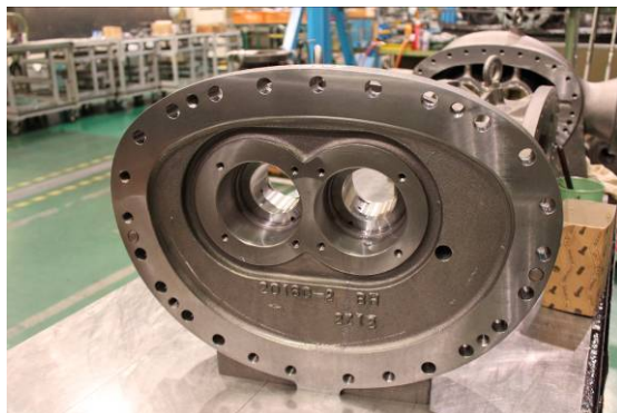
Photo 048 After Removal of Stop Rings and Main Bearings
