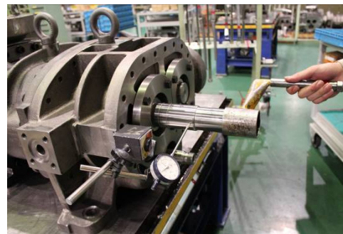
Photo 092 Measuring Runout of Shaft
