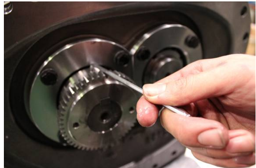
Photo 035 Removing the Driven Hub
