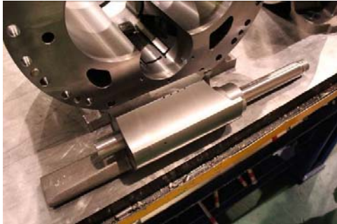
Photo 058 Unloader Slide Valve
