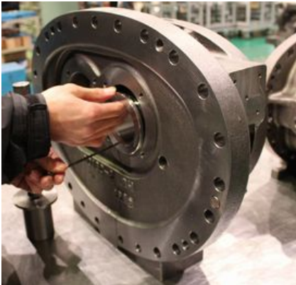
Photo 062 Attaching Main Bearing (High-stage)
