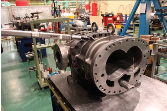
Photo 064 Fastening Low-stage Assembly with Bolts
