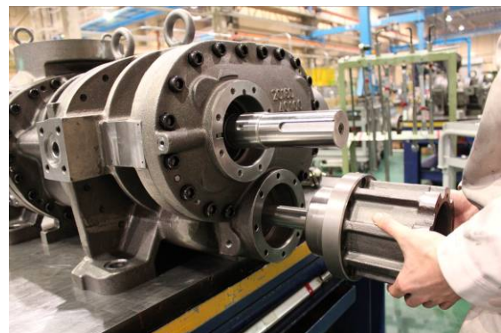
Photo 028 Removing Low-stage Unloader Cylinder
