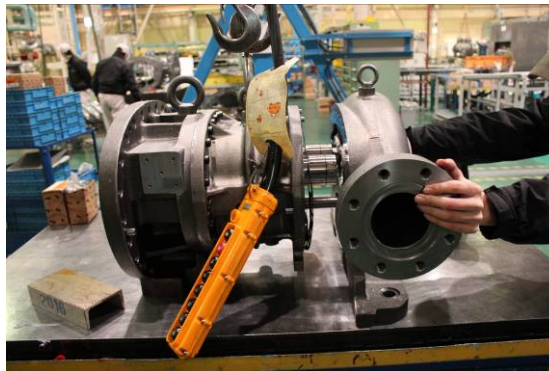
Photo 043 Pulling Out Suction Cover
