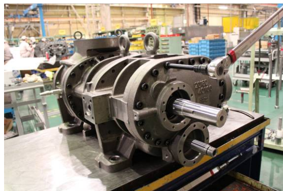
Photo 095 Tightening Bearing Cover
