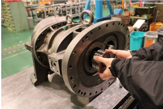
Photo 037 Pulling Out Thrust Bearing
