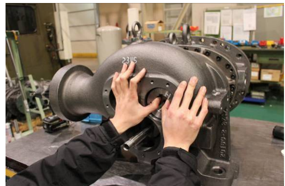
Photo 084 Attaching the Balance Piston
