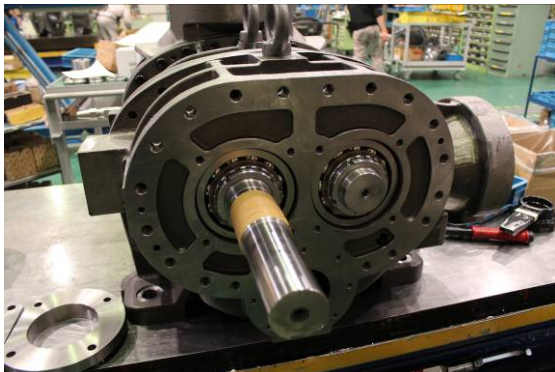
Photo 051 Thrust Bearing Glands are Just Removed
