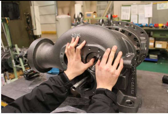
Photo 041 Pulling Out Balance Piston
