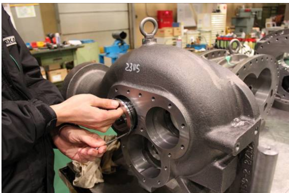
Photo 072 Attaching Side Bearing (High-stage)
